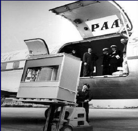
1960 Disc drive 1.1 tonne; 50 Mb
